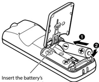
Insert the battery's negative terminal first.
