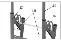
b. Pull back through 90° on the axle of the front triple wheel units so that the rear castors meet the ground and the vertical back rest of the sack truck now forms the horizontal bed of the platform truck.
