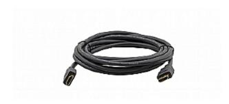
Kramer's C-MHM/MHM is a flexible high-speed HDMI cable with Ethernet. It is a high-performance cable with molded HDMI connectors at both ends that supports signals up to 1920x1200 @60Hz and HDMI Ethernet Channel, 12-bit Deep Color, x.v.Color™, Lip Sync, HDMI Uncompressed Audio Channels, Dolby TrueHD, DTS-HD, CEC.
