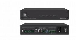
PA-240Z is a high-performance Hi-Z (70V/100V) and Lo-Z (4/8 $\Omega$ ) controllable power amplifier featuring balanced and unbalanced inputs and line-level output. This powerful amplifier is suitable for large-scale applications
