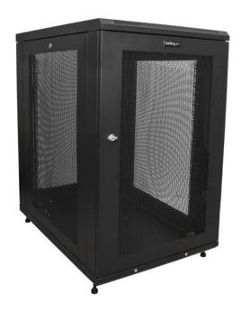
This server rack provides 18U of storage space in a sleek, secure cabinet for storing standard 19" rack-mount devices such as Dell, HP, and IBM servers, along with telecommunication and A/V equipment. The rack is compatible with EIA-310 compliant equipment and supports a total load capacity of 450 kg (992 lb.).
