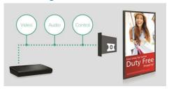
HDbaseT is a connectivity standard over a single CAT5e / 6 cable, converging uncompressed full HD digital video, audio signals.
