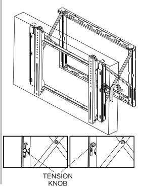
Note: Do not remove tension knobs.
