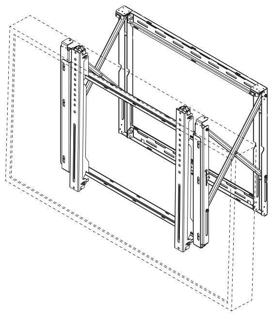
Max UL Load Capacity: 225 lb (102 kg)
