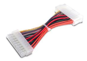
This 20 to 24-pin Power Supply Adapter features a 20-pin Female ATX connector as well as a 24-pin Male ATX connector, providing a cost-effective way to connect a 20-pin compatible motherboard to a power supply with a 24-pin connector, allowing the use of a newer 24-Pin Power Supply with an older 20-Pin Motherboard
