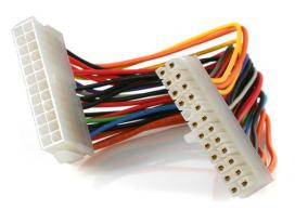
This 24-pin ATX 2.01 Power Extension Cable offers a male 24-pin ATX connector as well as a female 24-pin connector, allowing you to extend the length of an ATX power supply connection by 8in, providing enough cable slack to position the motherboard as needed in relation to the power supply without having to strain the ATX power connection.
