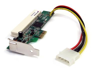
This PCIe to PCI Adapter Card lets you use low profile PCI expansion cards in a server or desktop motherboard PCI Express slot. Compliant with PCI Express Specification 1.0a and PCI Specification 2.2, the adapter card connects through a PCIe 1x slot to provide a low profile PCI slot in its place. A spare full size bracket for PCI Express card is also included for use in larger desktop or server PCI Express slots.
