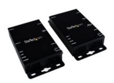
The ST121UTPHD2 HDM® over Cat5 Extender Kit can extend the audio and video signal output from an HDM®-equipped device by up to 330 feet (100 Meters), over a single CAT5 cable, or up to 165 Feet (50 Meters) over a single CAT6 cable. The extender supports full High-Definition video (1080p) and HD 3D, and also extends the accompanying digital audio signal.
