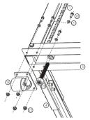
2. Stand the rack upright and install the included Cable Management Hooks in your desired locations as shown.
