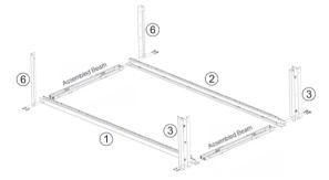
Using the remaining two Beams assembled in step 1, line up the other set of Left and Right Vertical Rails and fasten them to the Base and Top Brackets as shown.
