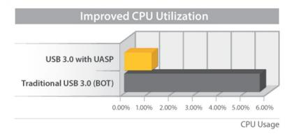
Test results were obtained using an Intel® lvy Bridge system, StarTech.com add-on USB 3.0 cards, a UASP-enabled StarTech.com enclosure, and a SATA III solid state drive.
