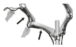
3. Use the Cable Clip (14) to secure the display cables to the pole.
