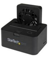
This USB 3.0 and eSATA docking station makes it easy for you to connect and swap your 2.5in or 3.5in SATA hard drives (HDD) and solid-state drives (SSD). The docking station also has a built-in fan that keeps your drives running at an optimal temperature for peak performance and longer drive lifespan.
