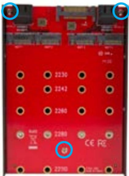
3. **(Only required if any of the drive installation screws and standoffs requires relocating)** Remove the screw holding the SSD standoff you wish to move, from the reverse side using a small Phillip's head screw driver (not included).
