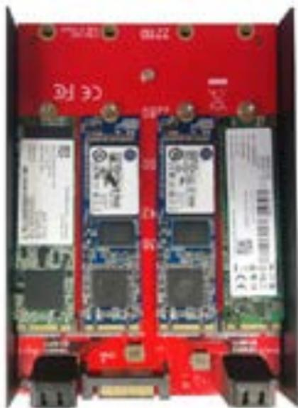
2. **(Only required if any of the drive installation screws and standoffs requires relocating)** Using a Philip's head screw driver, remove the three board mounting screws pictured below.
