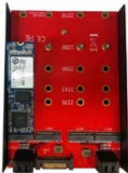
**Note:** The connector on your M.2 SSD is keyed so the drive will only fit one way.
