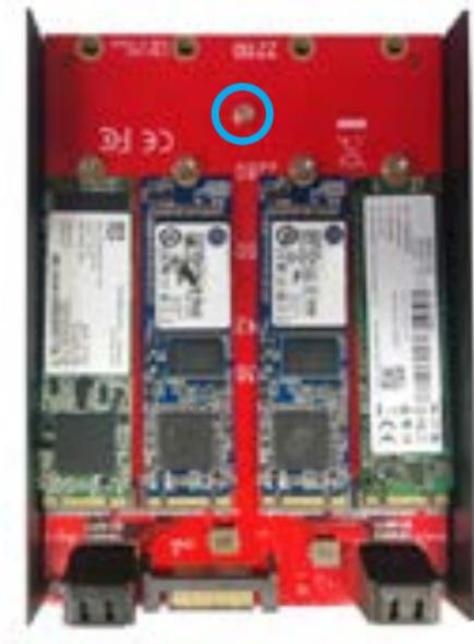
8. The SSD has now been installed, and is ready for system installation.
