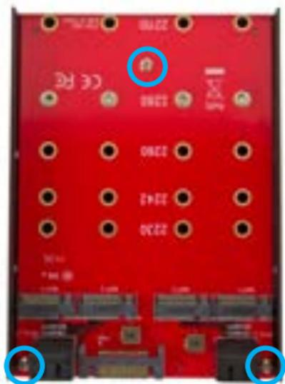
6. Slide the M.2 connector on the SSD into the M.2 receptacle connector on the 35524M2NGFF.
