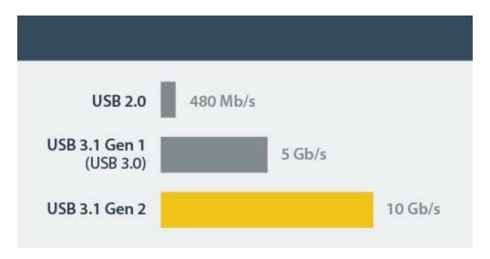
USB 3.1 Gen 2 gives you greater bandwidth and speed with file transfer rates of up to 10 Gbps - twice the speed of USB 3.0 (USB 3.1 Gen 1) technology. It lets you leverage the high performance of the latest SSDs and hard drives, while alleviating bottlenecks in your data transfers.
