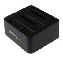
Get unprecedented performance and storage capacity with this USB 3.1 Gen 2 (10 Gbps) dual-drive docking station. It supports both 2.5" and 3.5" form factor solid-state and hard drives, with a high capacity storage capability of 12TB (6TB per drive).
