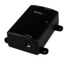
This Gigabit Power over Ethernet (PoE+) injector supplies power and data connectivity to a Gigabit PoE-compliant device using standard Ethernet cable, at distances of up to 100 m (330 ft.).
