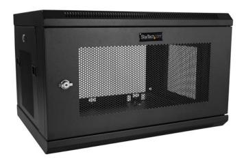
This 6U server rack cabinet lets you mount your EIA-310 compliant equipment to the wall. The enclosure features a mounting depth up to 16.9 in. and offers a maximum load capacity of 200 lb. (90 kg).
