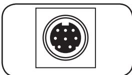
**Mini-DIN Serial Port:** Use this port to provide a direct terminal connection to a computer with a terminal emulation program. A serial cable (part number 73-1025) is included with the PDU. If you need to order a replacement cable, contact Tripp Lite Customer Support at 773.869.1234.
