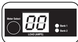
**Digital Load Meter (Ammeter):** The digital load meter displays the load in amps. It may be set using the Meter Select switch to display the PDU's total connected load (all 16 outlets-both LEDs illuminated), or the load carried by either the upper bank (Bank 1 LED illuminated) or lower bank (Bank 2 LED illuminated) of 8 outlet receptacles. For models with SNMP Network Card installed, press and hold the switch to display the IP address of the SNMP card in the PDU.
