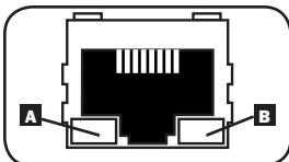
**Ethernet Port:** Use this RJ-45 jack to connect the PDU to the network with a standard Ethernet patch cable. The Link LED **A** and Status LED **B** indicate several operating conditions, as shown in the table below. Note: *This port is not compatible with PoE (Power Over Ethernet) applications.*
