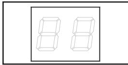
**Digital Load Meter (Ammeter):** The total electrical current drawn by connected equipment is displayed on the meter in amperes.
