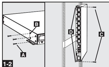
**1-3 Wall Mounting:** Use 3 screws **A** to attach each of the 2 shorter mounting brackets **B** to the PDU as shown. Mount the PDU to the wall by inserting 2 or more user-supplied screws **C** through the mounting brackets **D** and into secure mounting points.
