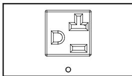
**NEMA 5-15/20R Output Receptacles (PDUMH20NET):** During normal operation, the output receptacles distribute AC power to connected equipment. When an outlet is live, the associated LED illuminates.
