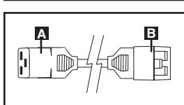
**AC Input Power Cord (Model PDUMH20HVNET):** The detachable cord has an IEC 60320 C19 connector **A** and an IEC 60320 C20 connector **B**.
