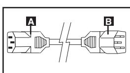
**AC Input Power Cord (Model PDUMH15HVNET):** The detachable cord has an IEC 60320 C13 connector **A** and an IEC 60320 C14 connector **B**.
