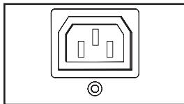
**IEC 60320 C13 Output Receptacles (PDUMH15HVNET & PDUMH20HVNET):** During normal operation, the output receptacles distribute AC power to connected equipment. When an outlet is live, the associated LED illuminates.
