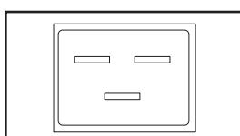
**AC Input Power Inlet (Model PDUMH20HVNET):** The IEC 60320 C20 inlet connects to the detachable AC Input Power Cord.
