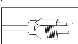
**AC Input Power Cord (Model PDUMH15NET):** The cord is permanently attached to the PDU and has a NEMA 5-15P plug.
