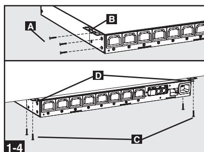
**1-5 Reduced-Depth Mounting:** Use 3 screws **A** to attach each of the 2 shorter mounting brackets **B** to the PDU as shown. Mount the PDU to a stable surface with the outlets facing upward by inserting 2 or more user-supplied screws **C** through the mounting brackets **D** and into secure mounting points.
