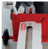
Adjustable width brackets to hold the box firmly in place.
