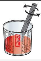
Remove the spray gun. Pull up on the tab and unlock the seal in a circular motion to remove the lid. Refill the cup with paint and reseal the lid.
