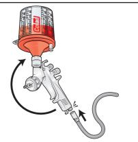
Tilt the spray gun forward and backward to release any air below the filter.
