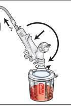
Install the Snap Lid System® adapter specific to your spray gun model with a Wrench #22. Keep the adapter installed on the spray gun.
