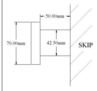
The SK15 Skip Lock is designed to fit skip lugs as dimensioned above.
