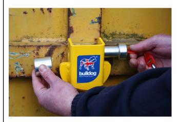
2. With the lock bolt in the unlocked position, insert it through the cover and lock it into the end cup by turning the key a quarter turn clockwise. Remove the key.
