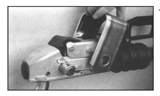
1. Lower Hitchlock over the front fixing bolt of the hitch head.
