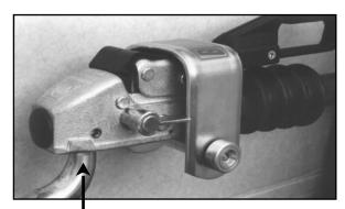
2. Insert the locking bolt through the two holes in the Hitchlock and push lock cup over end of locking bolt. Turn key 1/4 turn clockwise to lock and remove key.
