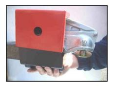
3. With the top box resting on the top of the handle of the hitch, position the bottom channel so both sets of holes line up.
