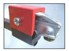
4. With the lock bolt in the unlocked position, insert it through the holes, place the cup over the end of the locking bolt and lock in position by turning the key a quarter turn clockwise.
