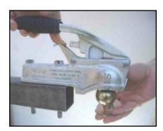
1. Insert the dummy ball when the trailer is unhitched by lifting the handle upwards, push the dummy ball into the socket and lower the handle. Insert the key into the lock and turn it a quarter turn anticlockwise, remove the lock bolt from the hitchlock and leave in the unlocked position.
