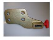
LC18 Wider than a standard car plate the LC18 is normally used on vehicles with an adjustable towbar or when there is limited ground clearance. For use with with Bulldog 200Q Stabiliser.
