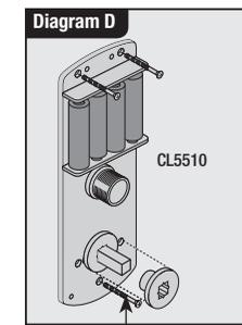
Alignment insert MUST be removed before completing installation.
