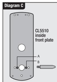
7 Screw the cable tube into the front plate, passing the cable through the tube. For doors less than 45mm (1 25/32") thick screw the tube all the way to the end of the thread. For doors more than 45mm (1 25/32") leave an appropriate amount of thread showing to accommodate ring nut. **Example:** For a 60mm (2 3/8") thick door leave 15mm (3/8") of thread showing.
