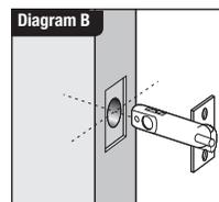
5 Fix the latch with the wood screws, with the bevel towards the door frame.
