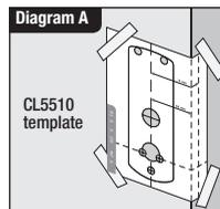
2 Keeping the drill level and straight, drill a 25mm (1") hole in the centre of the door edge to accept the latch.
