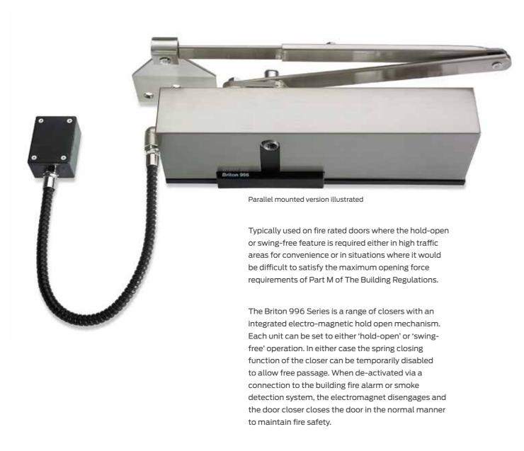
The Briton 996 Series is CE marked to EN 1154 and EN 1155 for electrically controlled closing devices, fire tested to EN 1634 and Certifire Approved for use on timber doors to achieve a 2 hour fire rating.
