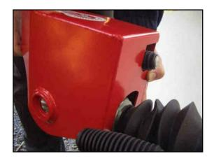
2. Tilt the rear of the red hitch lock cover back and "feed" the handle through the slot provided.
