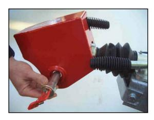
**4.** With the lock bar in the unlocked position, insert it into the red cover and push it into the lock housing. When in position, turn the key 1/4 turn clockwise to lock and remove key.
