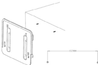
3. Attach the screws using wall plugs and put on the wall mount. The wall mount should be completely screwed together only after placement onto the screw heads.
