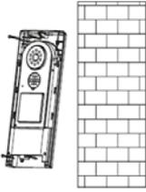
After finishing the wall mounting, put the door station back together to complete the installation.
