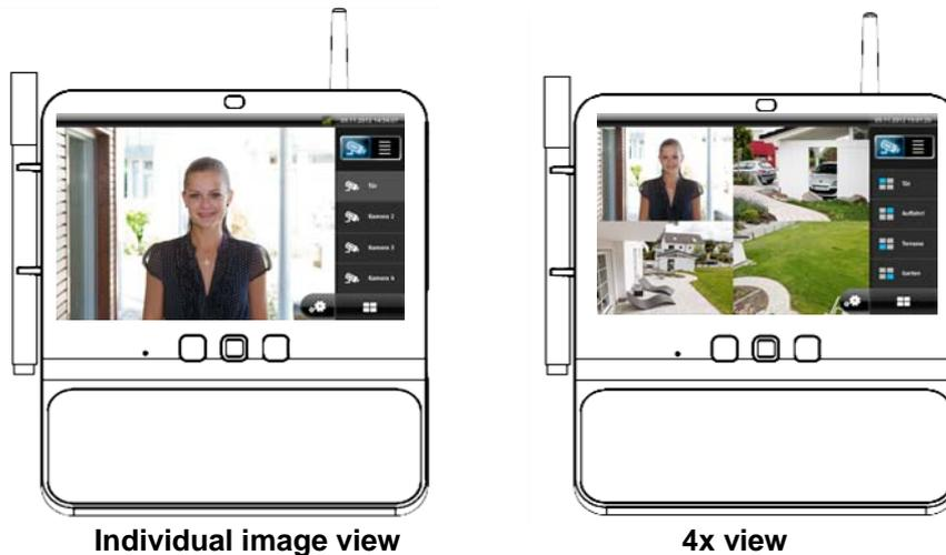
The Eycasa main unit has a touchscreen interface; all functions are operated by finger pressure on the appropriate button. In the live view, the following adjustment options and displays are available:
