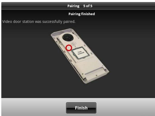
If the message “Video door station was successfully paired” appears, the pairing process is finished. The status LED goes out on your video door station, signaling readiness.
