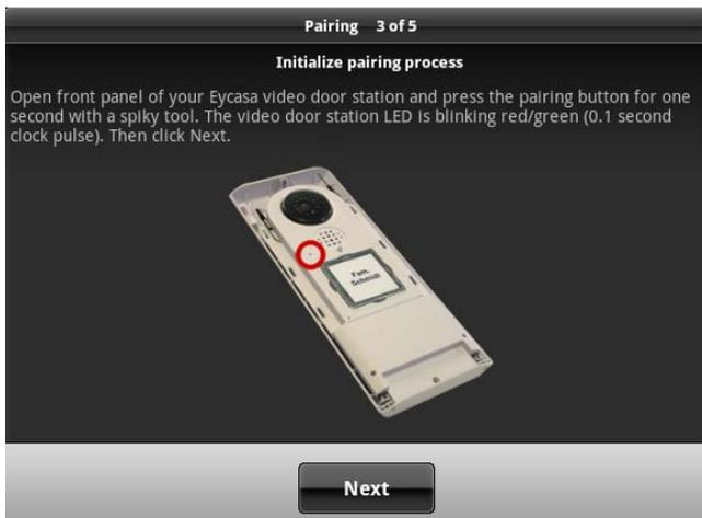
If your video door station is running on batteries, then you need to press the doorbell button once to wake up the device from standby mode. Now press the pairing button on your video door station. The status LED on your video door station flashes alternately red and green to indicate that the pairing process has started. The pairing process is active for 120 seconds. Press the "Next" button.
