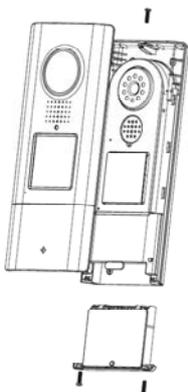
You can now open the plastic cover of the doorbell button and attach your nameplate. For labeling, you can use the included nameplate or the PDF template on the included CD.
