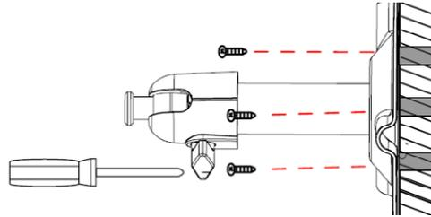
You can also swivel the mount by 90° into a particular position. First loosen the screw on the side and set the required angle. Then tighten the screw to secure the required position.
