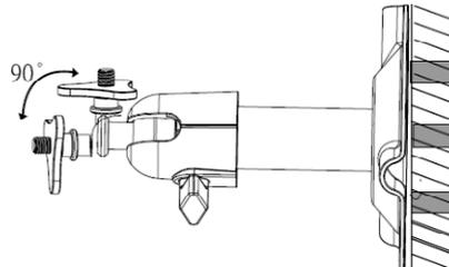
Screw the camera onto the mount and connect the power supply unit to the camera.
