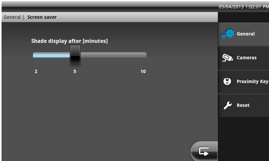
The screen saver is automatically activated after the set time if during this time there has been no user input on the touchscreen and no events on the main unit. The monitor dims in this mode, but the system functions are still active.
