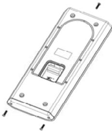
If you are operating your video door station with a permanent power supply (bell transformer), remove the cover of the terminal connector on the rear of the device.
