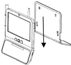
2. Put the wall mount into the desired position on the wall and mark the drill holes. The distance between the two holes is 102 mm.
