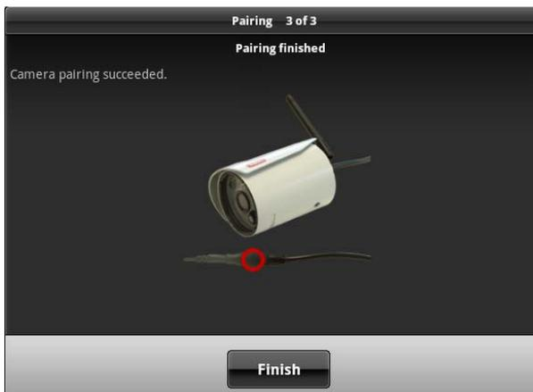
Once the message "Camera pairing succeeded" appears, you can release the pairing button. The pairing process is completed. If an error occurs during the process, repeat the previous pairing steps.
