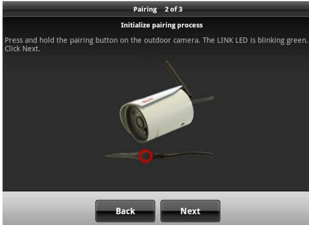
Follow the instructions on the screen and press and hold the pairing button on the power cable of the camera. The link LED of the camera starts to flash. Now press "Next" without releasing the pairing button.
