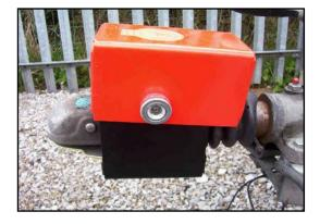
**6.** Push cup over end of locking bolt Turn key quarter turn clockwise to locK and remove key.
