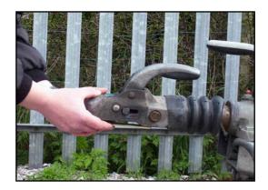
**1 & 2.** Insert dummy ring plate to trigger the handle into its lower position.
