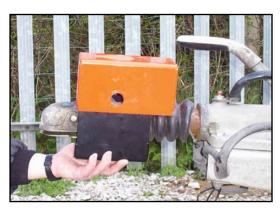
**4.** Lower the top box noting that the extension fits towards the rear of the handle as shown.
