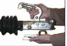
1. Insert dummy ring plate. If hitch handle is in raised position the plate can be used to release handle.
