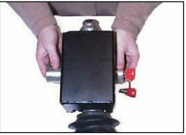
**6.** Push cup over end of locking bolt. turn key quarter turn clockwise to lock and remove key. Fit red plastic cover.
