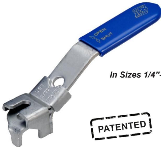
The **RuB** lockable handle is made of strong Geomet® carbon steel and designed to discourage tampering. The **RuB** locking device covers the top nut of the valve making removal impossible without a key. Easy to install on valves in the field, the **RuB** lockable handle will lock s.93 **RuB** valve the closed position only in compliance with OSHA (USA) safety requirements, while other **RuB** valves can be locked in both the open and closed positions.
