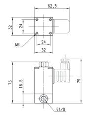
The G1/8 N.C. (closed) or N.O. (open) 3/2 - way solenoid valves are particularly suitable for operating single-
