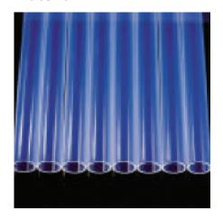
FEP is similar to PTFE with regard to excellent dielectric properties; chemical inertness; toughness at low temperatures; low coefficient of friction; non-stick properties & weatherability. FEP has a higher degree of transparency and a greater modulus of elasticity at low temperatures than PTFE. As with all fluoropolymers, FEP tubing can be steam cleaned or chemically sterilized according to all industrial standards & is produced from FDA approved raw material.
