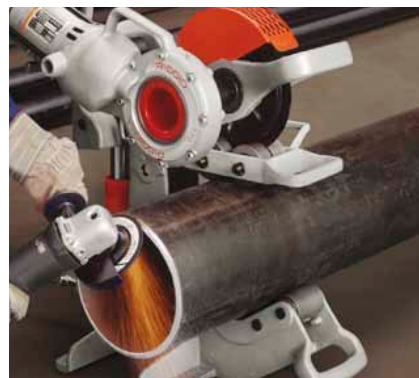
Model 258 with Pipe Roller in use for beveling. Two operators are recommended for this operation
