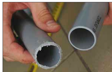
Cut with a hacksaw (left) versus the P-TEC 3240 (right).
