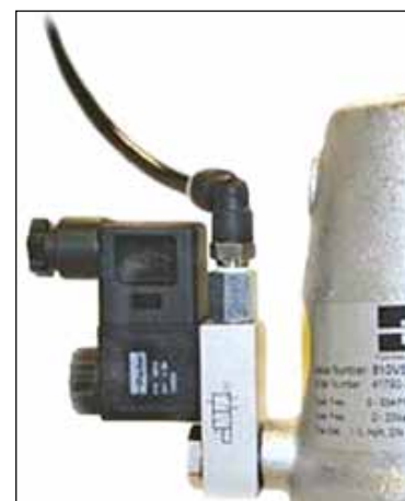
Banjo Valve Mounted to the valve
