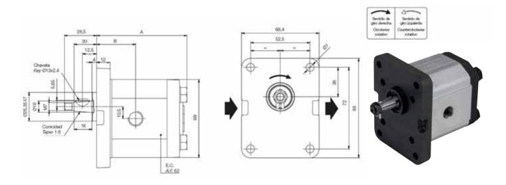
Clockwise rotation, 1:8taper shaft, 4bolt European flange, BSP ports
