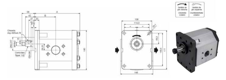
Clockwise rotation, group 3.5 taper shaft, group 3.5 4bolt flange, SAE ports
