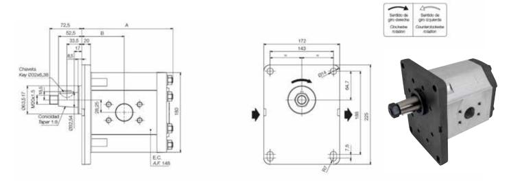
Clockwise rotation, group 4 taper shaft, group 4 4bolt flange, SAE ports
