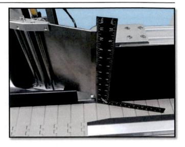
If the peel plate is not perpendicular to the conveyor loosen the mounting screws and nudge the plate up or down to square it up. When the plate is square tighten the mounting screws. There is some pressure on the peel plate so make sure the mounting screws are snug.
