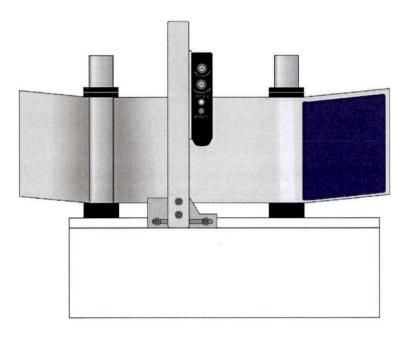
Pull a section of the web with labels through the sensor and confirm that the red LED illuminates when the sensor sees a label and turns off when the sensor sees the gap between labels. If you have an irregular shape label make sure that the sensor only sees the gap between labels rather than some point in the middle of the label.
