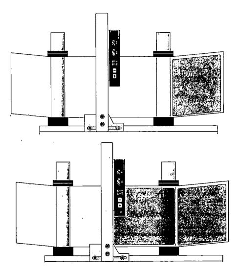
Pull a section of the web through the sensor so that the sensor is reading a label. Press the "+" button and the yellow LED will come on. Move the web back and forth so that the sensor reads a gap between labels. The yellow LED should go dark when the sensor sees a gap between labels.
