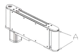
op and bottom tension screws should be belt top to bottom. Check belt tension by ith the pressure plate. The bottle should roll vrap belt without climbing or diving.
