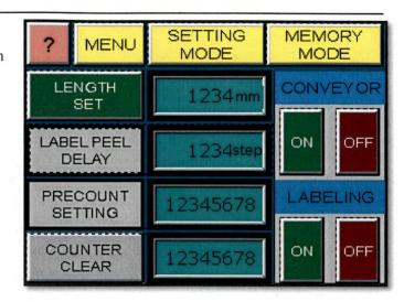
The number to the right of the length set button will increment as the web advances. The number resets to zero each time a gap between labels is detected by the label sensor.
