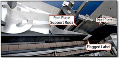
The labels must be outside the peel plate support rods and outside of the pinch roller cover as shown in these pictures.
