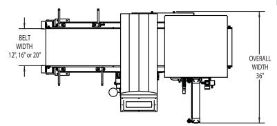
Example Model pictured shows a metal detector head on a Flex Conveyor with Pusher Reject. Overall widths may vary based on reject option selected.
