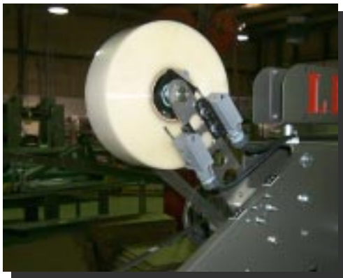
figure 20-1. Top Tape Supply Sensors
