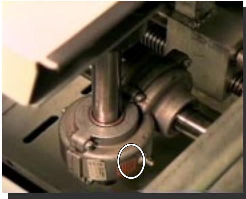
figure 19-1. Zerk Fitting on Tolomatic Gearcase
