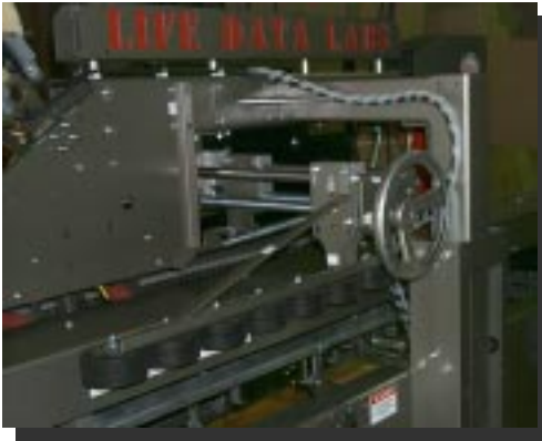
figure 25-1. Adjustment Handwheel for Side Compression Rollers
