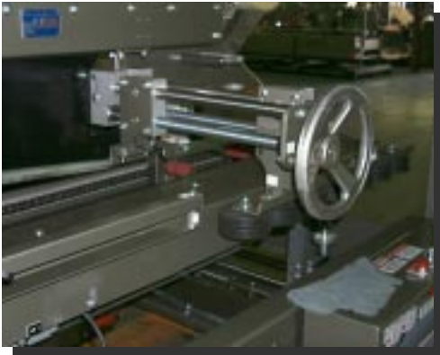
figure 25-2. Adjustment Handwheel for Top Major Flap Folders
