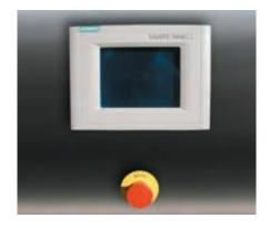
Touch screen interface with user-friendly input, storage and monitoring functions and emergency stop.
