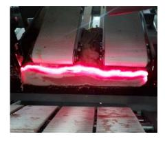
Rapid real-time scanning at 97% accuracy to the human eye. Grading and defect recognition as standard
