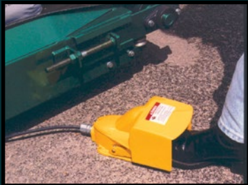
Operator foot switch leaves hands free for bag placement
