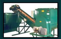
Incline conveyor for loading into various machines
