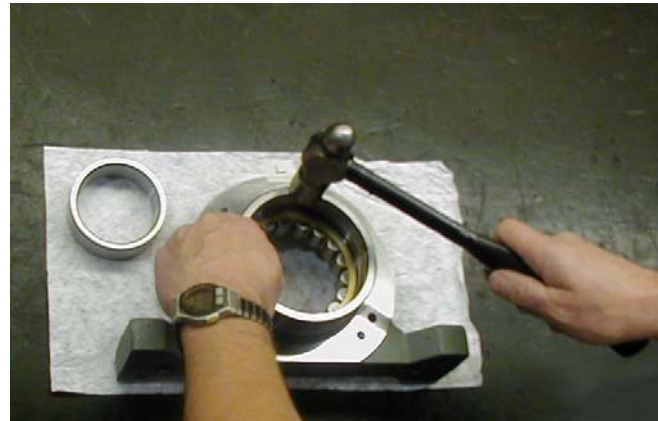
TAPPING BEARING INTO PILLOW BLOCK
