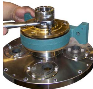
Figure 5-10 Main Bearing Installation Details
