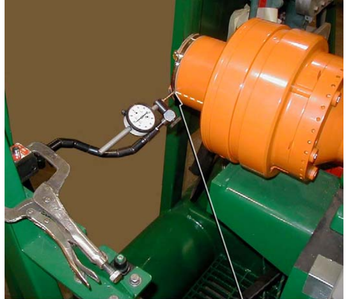
PLUNGER POSITIONED AT HORIZONTAL CENTERLINE OF GEARBOX
