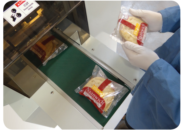
The standard FW 400F is equipped with print registration capability with precision control for indexing pre-printed films.
