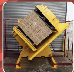
The 180 degrees of rotation makes pallet exchange quick and simple.
