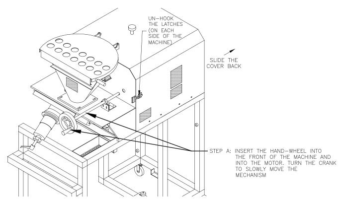
B. ONCE *PIN A* HAS BEEN REMOVED, TURN THE HAND-WHEEL SO THAT THE SPRING ASSEMBLY IS MOVING AWAY FROM THE CYLINDER. WHEN THE PISTON ITSELF BEGINS MOVING (WHEN THE SPRING ASSEMBLY HAS REACHED THE END OF ITS TRAVEL AND STARTS TO COME BACK) A SECOND SET OF HOLES WILL COME INTO ALIGNMENT AT THE CENTER OF THE CONNECTING ROD.
