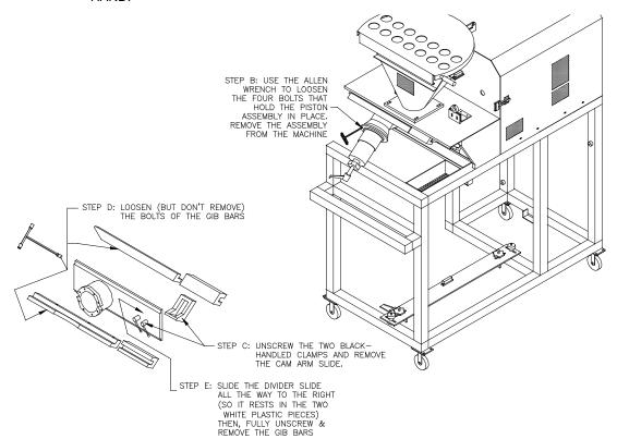
D. ONCE THE CAM ARM HAS BEEN REMOVED, USE THE 9/16 SOCKET ON THE LONG END OF THE T-HANDLE TOOL TO LOOSEN THE 4 NUTS HOLDING THE UPPER GIB BAR IN PLACE, AND THE 3 NUTS HOLDING THE LOWER GIB BAR. **DO NOT, HOWEVER, REMOVE THE GIB BARS AT THIS TIME.**
