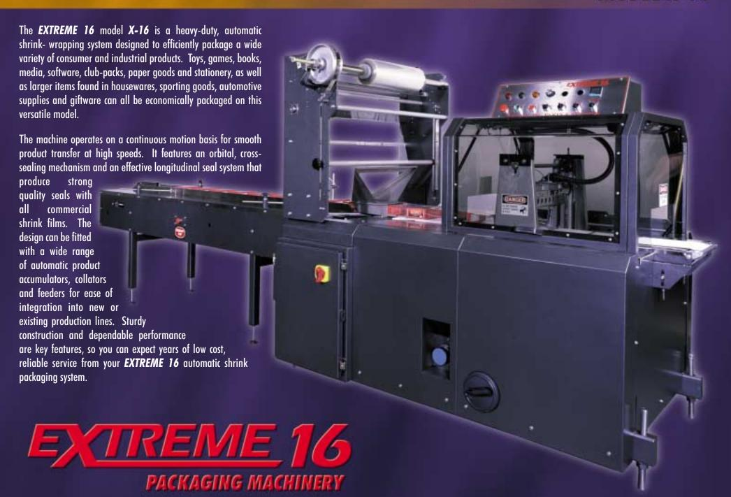
Introducing the **EXTREME 16 SERIES** Horizontal Form/Fill/Seal Wrappers. These heavy-duty wrappers are designed with versatility and multi-shift operation in mind. The proven mechanical design translates into straightforward operation and maintenance simplicity.
